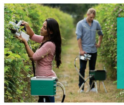
The LI-6400XT set the standard for portable photosynthesis systems. Now, the completely new design of the LI-6800 sensor head includes refinements to the gas analyzers, flow path, and temperature response as part of Rapid Sensing<sup>™</sup> Technology. Many LI-6800 advantages are due to this innovative new design.
